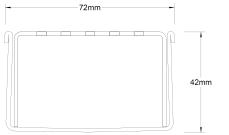
Grates longer than 1500mm supplied in sections. Tile Inserts longer than 1200mm supplied in sections. Channels over 3000mm supplied in sections with joiner. +/-2mm tolerance on
