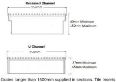
Grates longer than 1500mm supplied in sections. Life Inserts longer than 1200mm supplied in sections. Channels over 3000mm supplied in sections with joiner. +/-2mm tolerance on dimensions.
